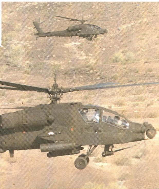
Below: Two fully armed Apaches on a training mission over the desert. Note how far the main landing gears hang down when unloaded. On the ground they are soft and spongy.
