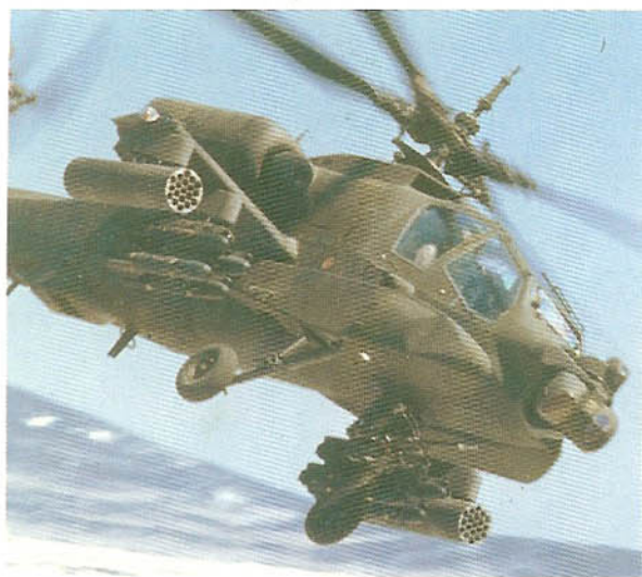
Above: This view gives a clear indication of the Apache's weapons and sensors. The PNVIS (pilot's right vision sensor) above the nose is swivelled to look at the photographer, and via the IHADSS could aim the gun at him on a dark night.
