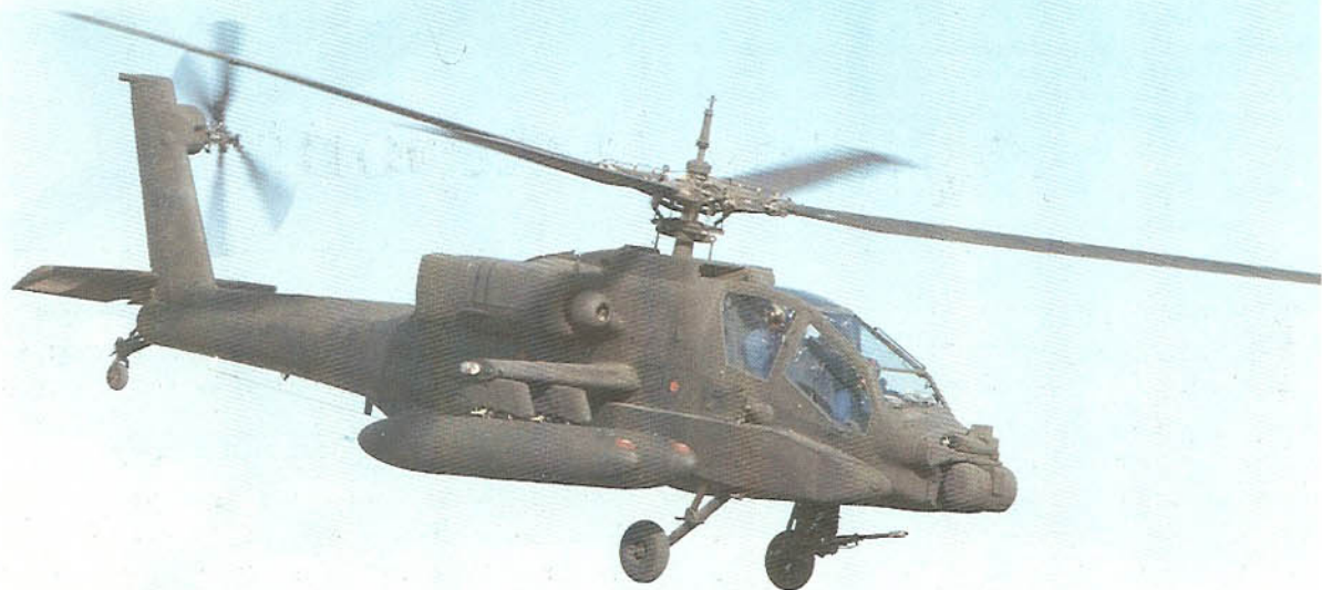
Above: McDonnell Douglas Helicopter test pilots departing on a simulated long-range deployment mission in ferry configuration with four auxiliary tanks. These extend range from 260nm (482km, 300 miles) to 918nm (1,701km, 1,057 miles).
