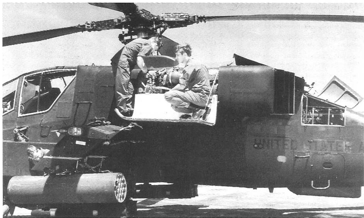
Above: Line maintenance on a US Army Apache, showing the excellent all-round access to the reliable T700 engines. Most of the bulk of the cowls is taken up by the IR suppressed jetpipes.
