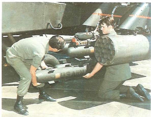
Left: From the outset of its operational career the primary anti-tank weapon of the Apache has been the hefty Hellfire missile, one of which is here being loaded by two crew members into a lower inboard launch rail. Missile weight is 101lb.
