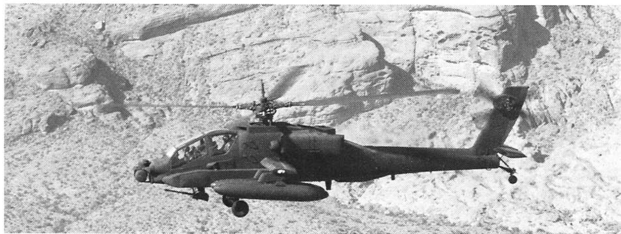
Above: This Apache demonstrated self-deployment (from the USA to Europe, if necessary) by making flights of more than 1,100 miles (1,770km) with four 230 US gal external tanks.
