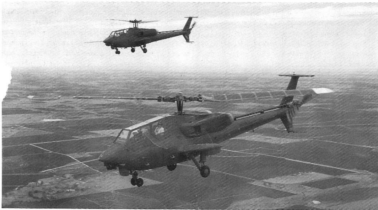
Below: The two prototypes of Bell's rival YAH-63 losing design which, among other things, put the pilot in front of the gunner and also featured a tricycle-type landing gear.
