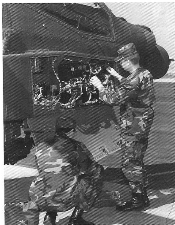
Above: Probably destined soon to be instructing others, these were among the first troops to specialize in the complicated avionics. These line-replaceable units are in the right-hand bay.
