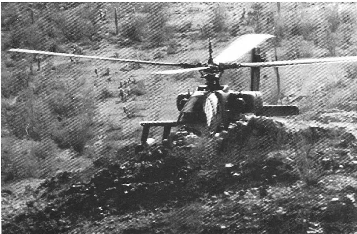
Above: In typical "hull down" position an Apache is hard to see or destroy. But as it has no mast-mounted sight, it is blind and impotent here until it exposes itself.
