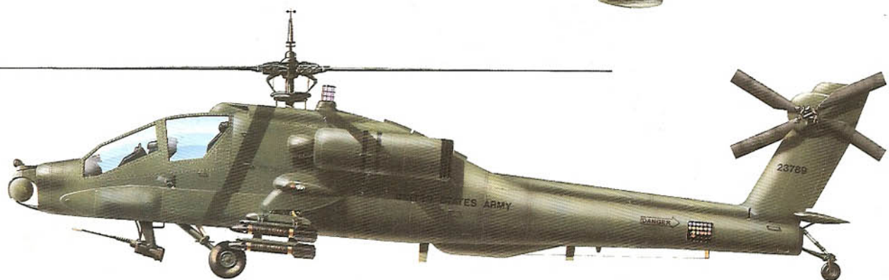
Above: Left-hand side elevation of an AH-64A Apache fitted with the ALQ-144 IRCM turret but with no FFAR rocket launchpods outboard of the quadruple Hellfires. Nose sensors are aligned fore and aft, as they normally are when inoperative.
