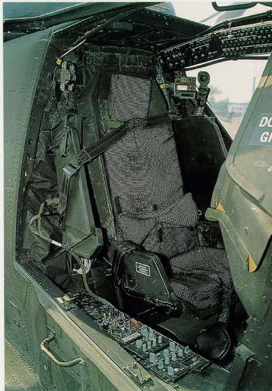
Above: The pilot's circuit breaker panel, located overhead on the left in the rear cockpit.
