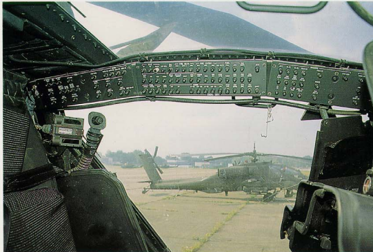
Above: The pilot's circuit breaker panel, located overhead on the left in the rear cockpit.
