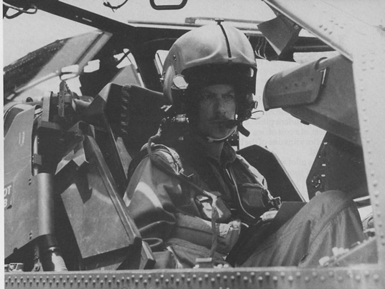
The TADS/PNVS turret and 30mm cannon can be slaved to the movements of either the pilot or copilot/gunner by a pair of Sensor Surveying Units (SSU) that are placed on the upper arm wings of each crew member's seat. The SSU generates IR beams that sweep the crew stations and feed position data to the Sight Electronics Unit (SEU). (McDonnell Douglas)
