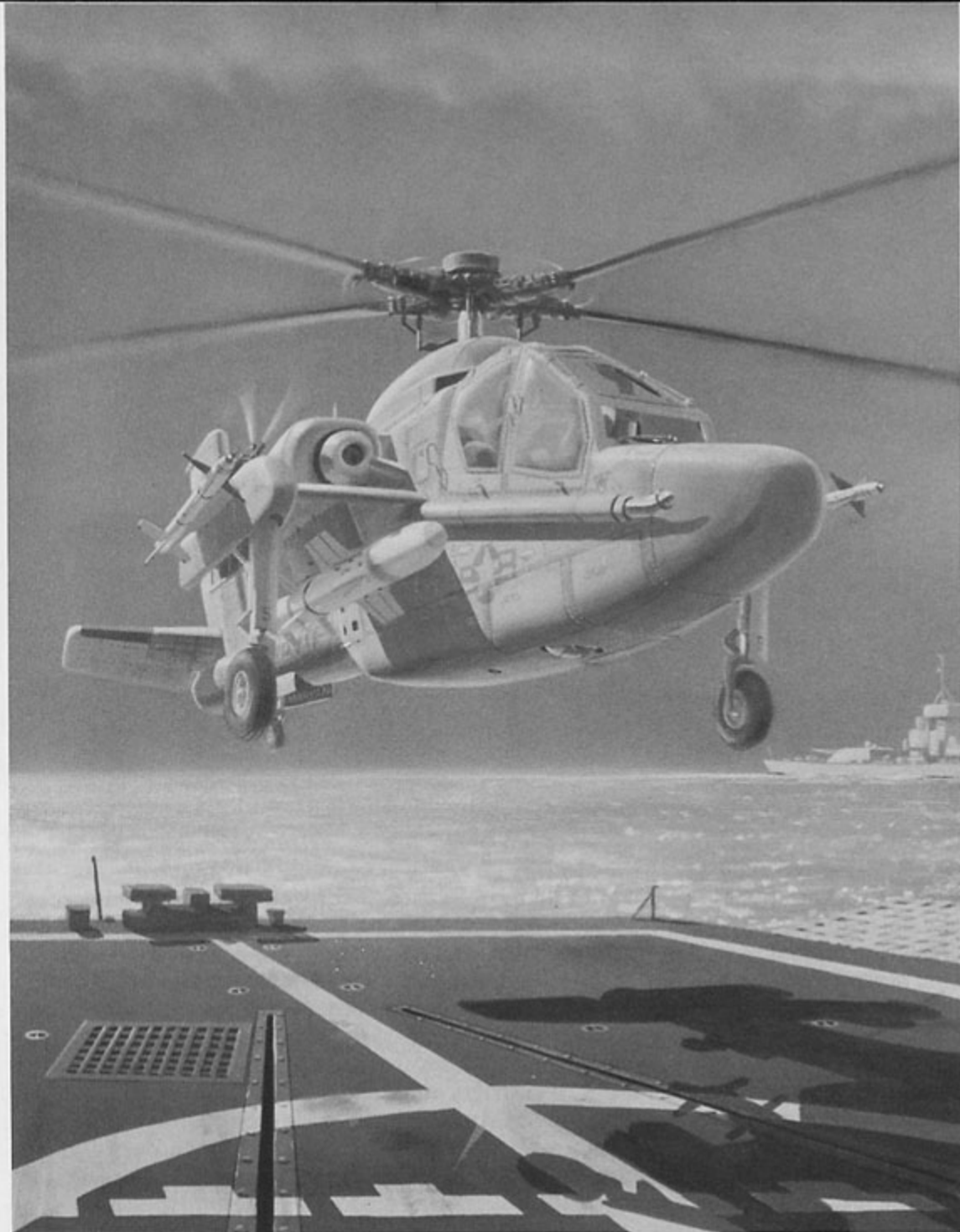
The final proposal for the Sea Apache calls for a deepened fuselage, a further modification to the nose section to incorporate a radar from an F/A-18 Hornet, and an inflight refueling probe. The projected missions for the Sea Apache include; anti-ship, anti-air, combat search and rescue escort, naval gunfire spotting and forward air control. (McDonnell Douglas)
