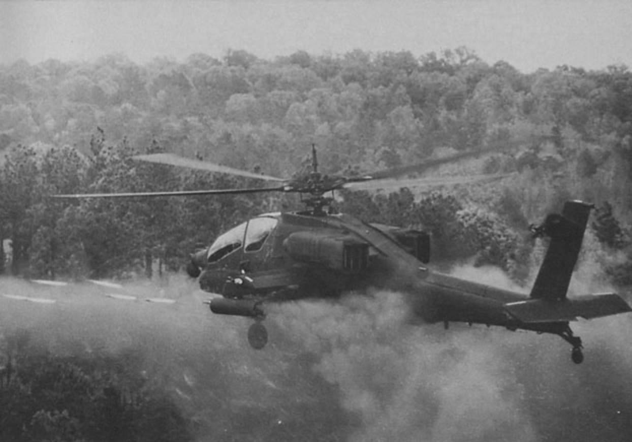
An AH-64A is enveloped in a shower of fire as it launches a salvo of 2.75 inch FFAR rockets during a live fire exercise on the Fort Rucker, Alabama firing range. The circular object just behind the rotor mast is the Disco Light IR Jammer. (U.S. Army)
