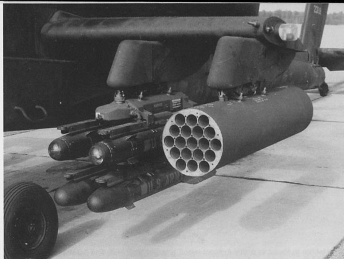
The stub wing pylon of an AH-64A armed with four Hellfire missiles and two Hydra 70 (LAU 61 A/A) 2.75 inch rocket launchers. The 2.75 inch rocket launcher weighs seventy-nine pounds empty and has a capacity of nineteen 2.75 inch folding fin aerial rockets (FFAR). (Author's collection)
