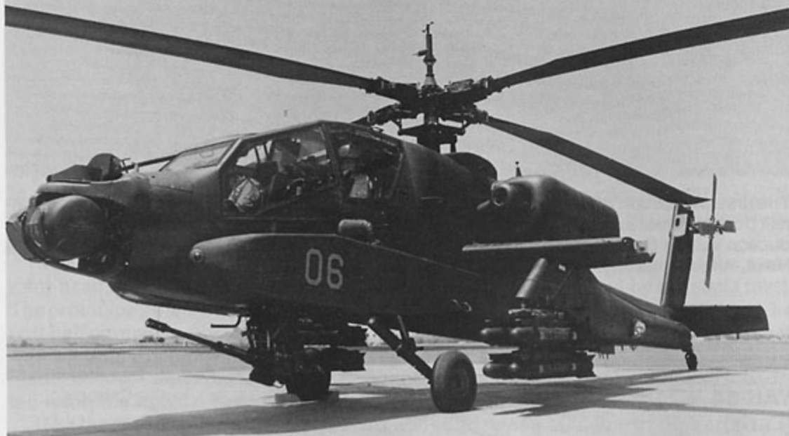
The sixth YAH-64 prototype (AV-06 77-23259) was the first to be fitted with the low mounted stabilizer. AV-06 was also fitted with a production TADS/PNVS nose turret, an Air Data Sensor (ADS) probe on the rotor mast above the blades, and extended side sponsons. (Rockwell)
