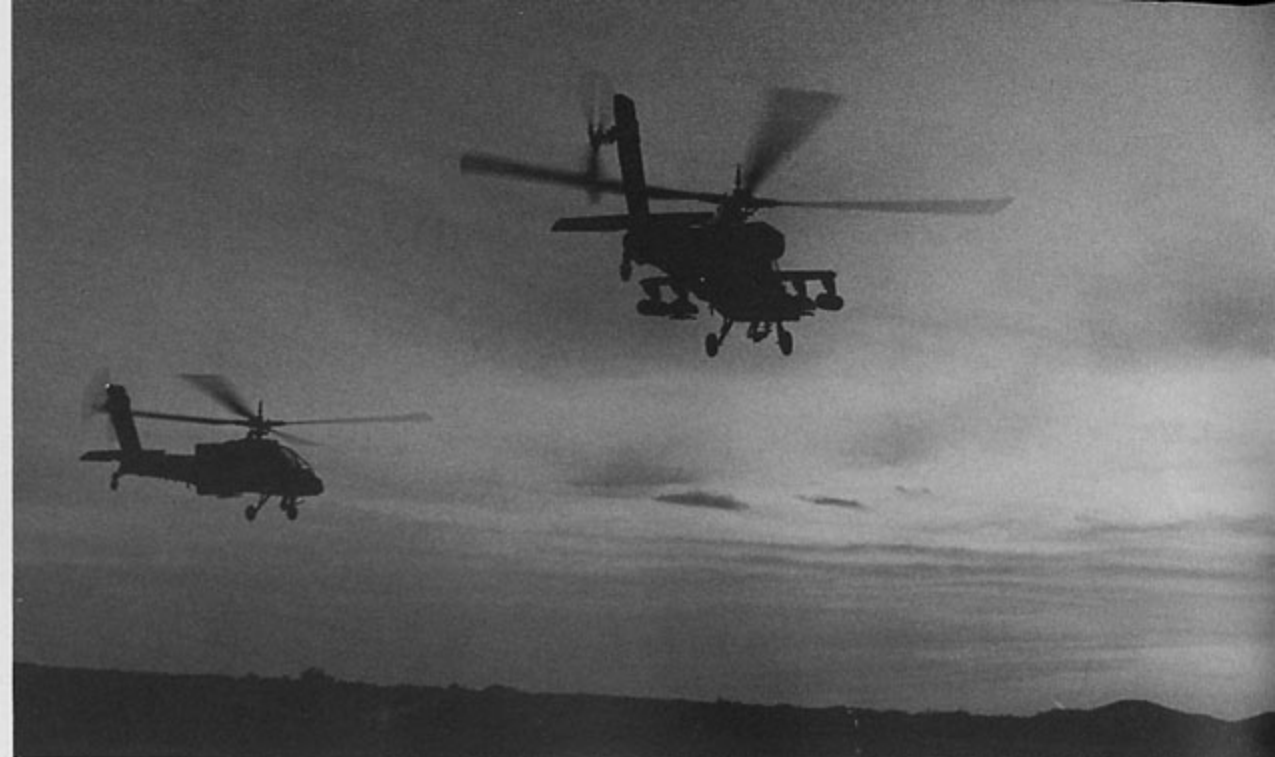
The Apache is routinely flown at night (and in bad weather) using the Pilot's Night Vision Sensor (PNVS) for navigation. Apaches usually work in hunter-killer teams with either another Apache or an OH-58 Kiowa scout helicopter. (McDonnell Douglas)
