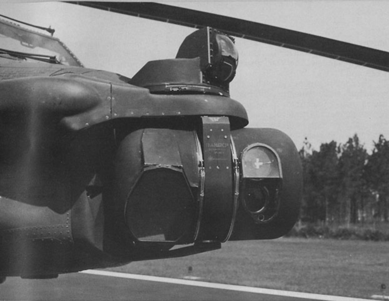
The nose of the AH-64A houses the TADS/PNVS turret. TADS is an acronym for Target Acquisition Designator System, while PNVS stands for Pilot's Night Vision Sensor. The TADS occupies the lower section of the turret while the PNVS is mounted above it. (Martin Marietta)
