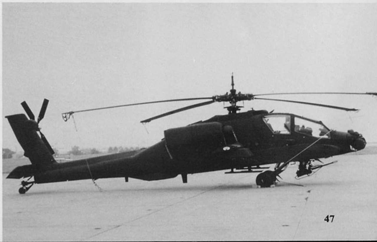
The main rotor blades of this Apache have been secured by tie downs to prevent the wind from causing the blades to flap. The tie down system consists of nylon bags that slide over the rotor tips and nylon lines that run from the rotor tips to the fuselage, securing the rotors in place. (China Clipper Photo)
