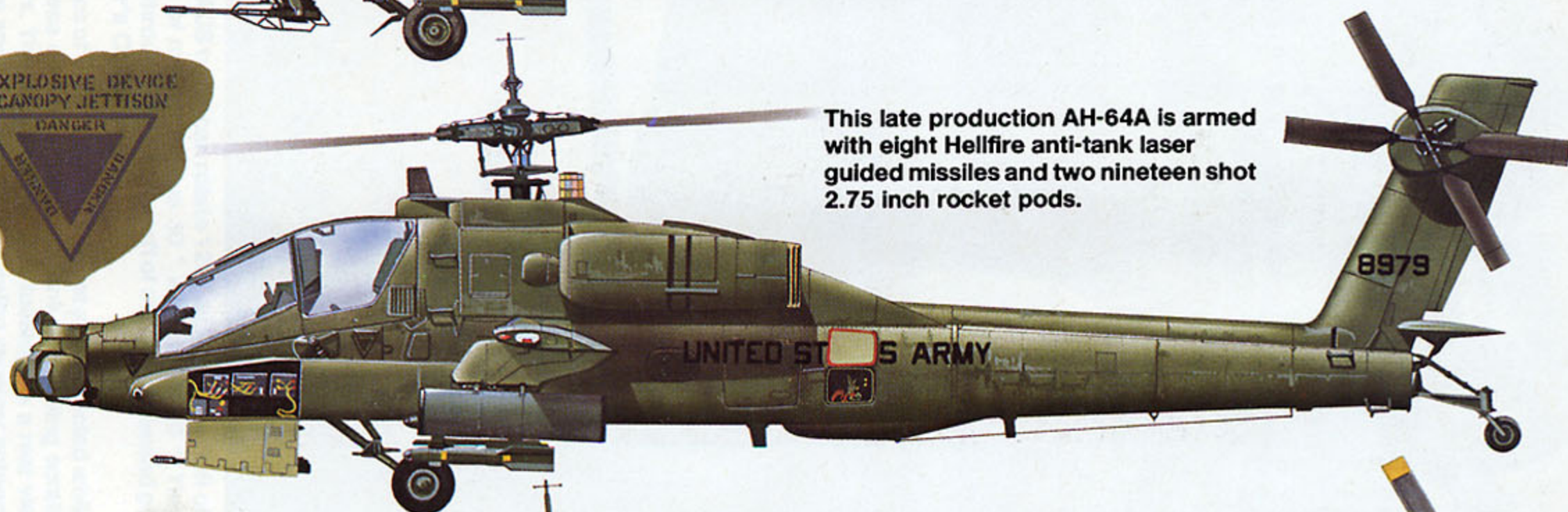
Configured with four 230 gallon underwing fuel tanks, the Apache has an unrefueled range of 1,175 miles. This Apache (83-23789) flew with one stop from Mesa, Arizona, to Fort Rucker, Alabama, during 1985.
