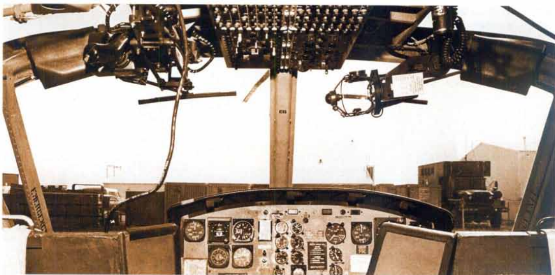
▼ A photo of the cockpit. An XM-60 sight of the M-6 armament system in stowed position under the cockpit ceiling on the right is visible. / Bell
