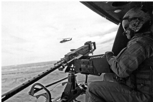
▲ A gunner of the US Marine Corps fits the ammo box to the GAU 21A machine gun during a patrol flight near Haditha in Iraq. The GAU 21A has the caliber 12.7 mm, theoretical rate of fire 950–1100 rounds per minute and maximum practical range of 1850 meters. It can be fed from 100, 300, and 600-round ammo boxes. / US Marine Corps
