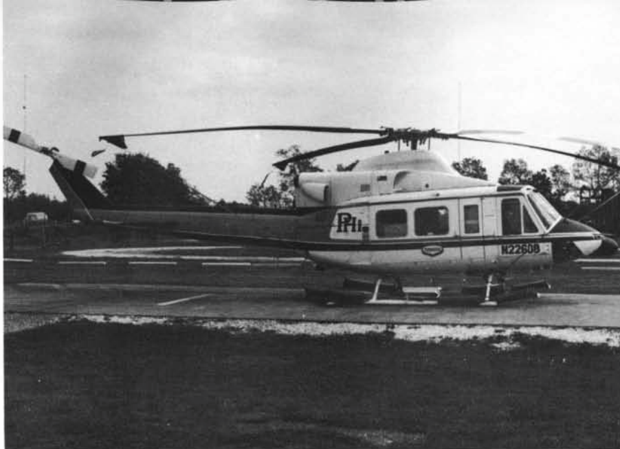
(Above Left) Belonging to Petroleum Helicopters Inc (PHI), this Bell 412 has float gear attached to the skids and weather radar mounted in the nose. The four bladed rotor has Red and White bands on its top surfaces. (Boyd Waechter)
