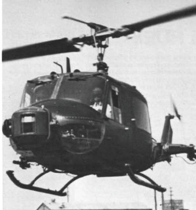
(Above) A 'FLIR' equipped UH-1M armed with flash suppressor-tipped M-134 mini-guns. (US Army)
