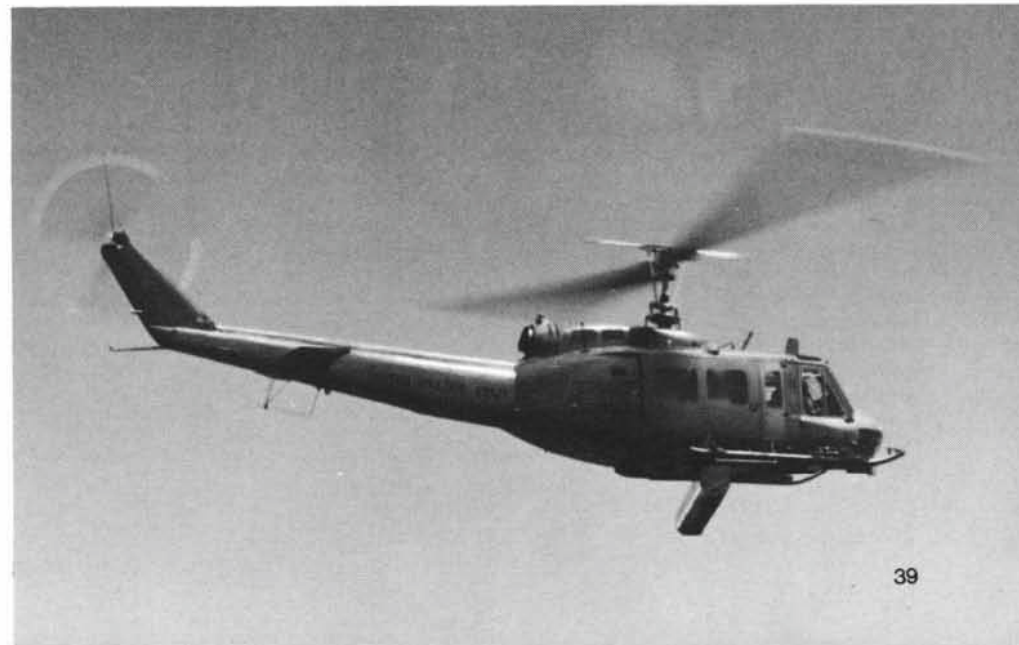
(Below) The skid is retracted and the SOTAS gear has been rotated into an operational position. (Bell)
