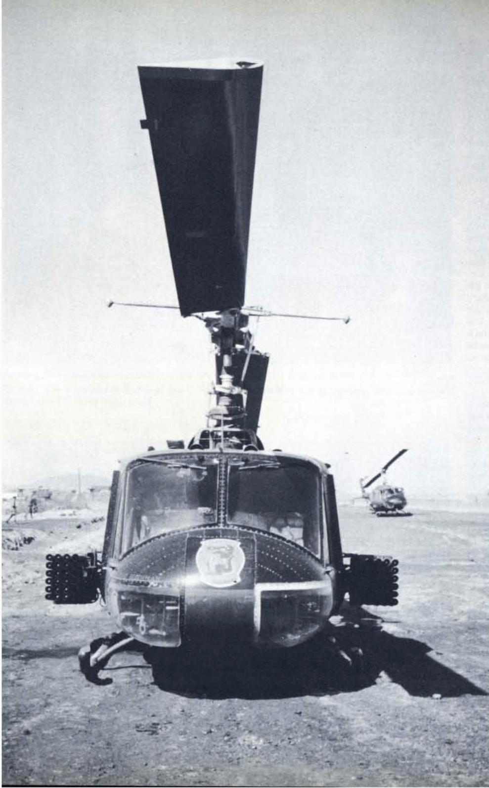
(Above) UH-1C HOGHEAD of Cobra V carrying twelve rocket tubes on each side and the nose mounted 40mm automatic grenade launcher. (E. Schwanebeck)
