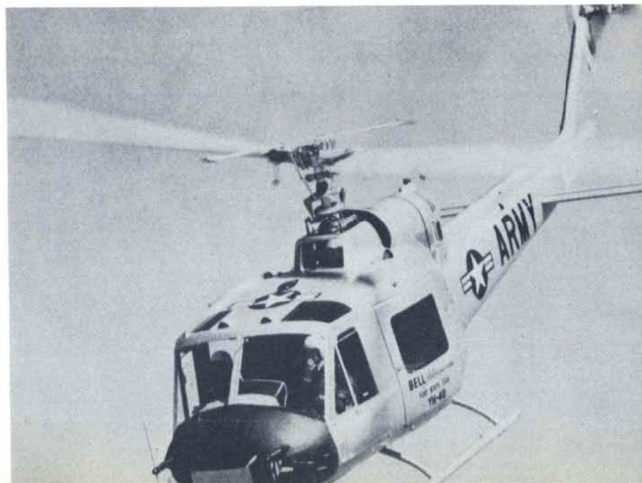
(Below) This YH-40, one of six evaluation machines built, clearly exhibits the significant improvements made over the XH-40 prototype — including the addition of the Bell-developed stabilizer bar mounted above the main rotor, a redesigned air intake and transmission cowling, and the relocation of the synchronized elevators to a more forward position on the tail boom. (Bell)
