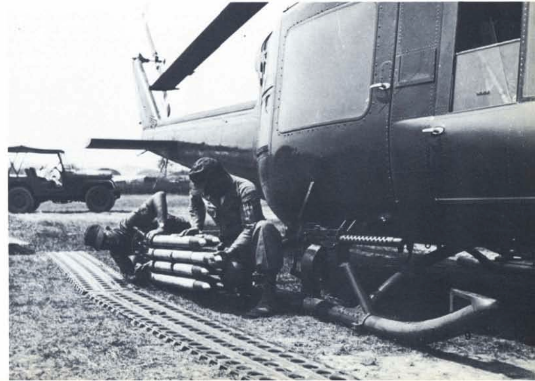
(Below) A 2.75 inch rocket installation is added next to the .30 caliber machine gun on this UTTC UH-1A at Tan Son Nhut, South Vietnam.
