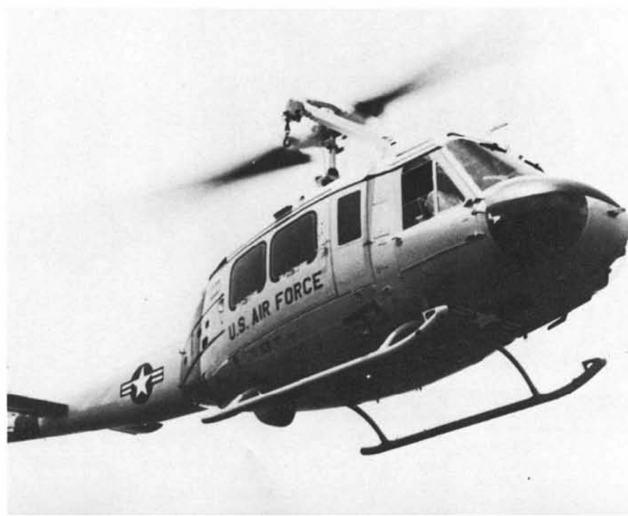
(Below) This HH-1H has its rescue hoist in the deployed position and carries a weather radome on its aft belly. The US National Insignia is painted on the lower surfaces along with RESCUE which is painted in Black. (US Air Force)
