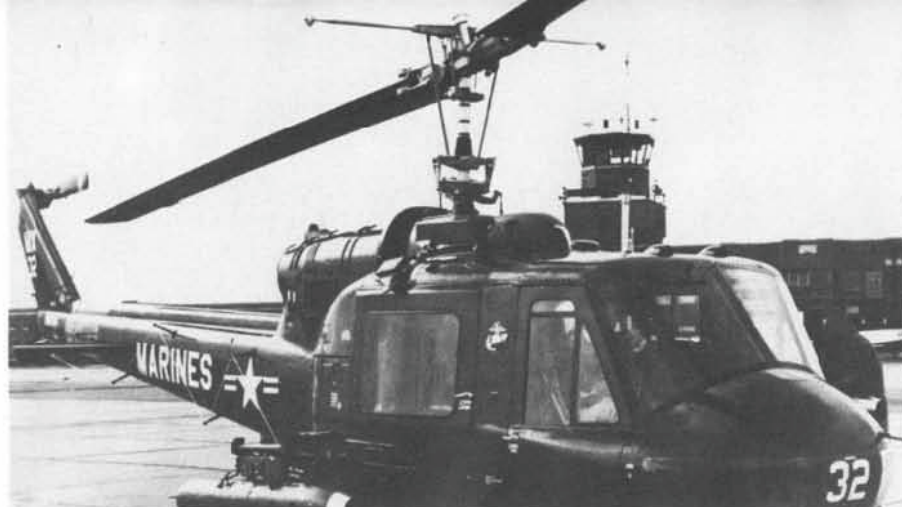
(Above) B model characteristics identify this UH-1E as one of the initial production batch examples. This 'Echo' Huey of HM-1 (Helicopter Development Squadron) at Quantico carries an unusual mixture of weapons, an XM-6 and XM-18 encased minigun, which was briefly tested on the UH-1B and was used operationally for a short time on the AH-1G Cobra. A USMC emblem is attached to the door post. (Bell)
