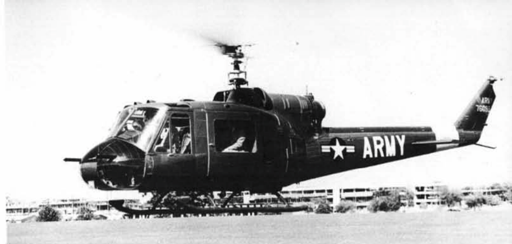
(Above) The fifth HU-1A to be built is being put through her paces for onboard officials. The A model is easily distinguished by its short rotor mast which would be lengthened 13 inches on the later UH-1B. (Smithsonian Institution)
