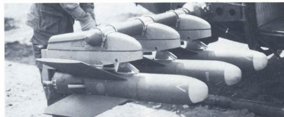
(Below) XM-22 anti-tank wire guided missile system mounted three missiles on each side. (Bob Steinbrunn)
