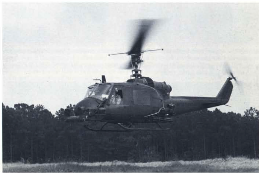
(Below) UH-1M Huey testing the Iroquois Night Fighter and Tracker (INFANT) system at Fort Rucker during 1969 prior to being deployed to Vietnam. (Defense Department)
