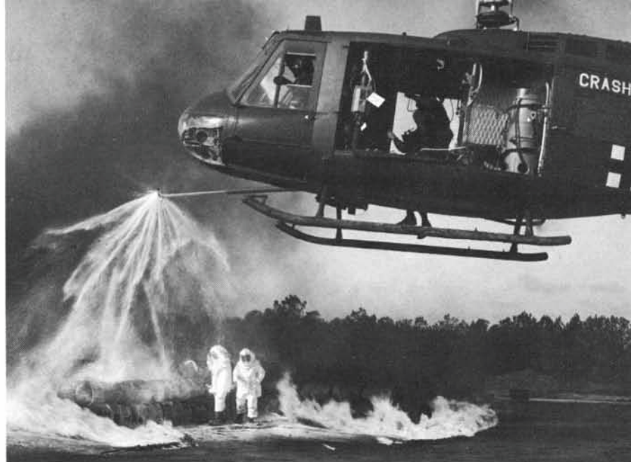
(Above) Fire fighters enter a mock crash area while a US Army HH-1D Crash/Rescue Huey creates a passageway with a 'light water' solution. In the cargo area can be seen the light water container and rescue hoist. Pope AFB, NC in January of 1972. (US Army)
