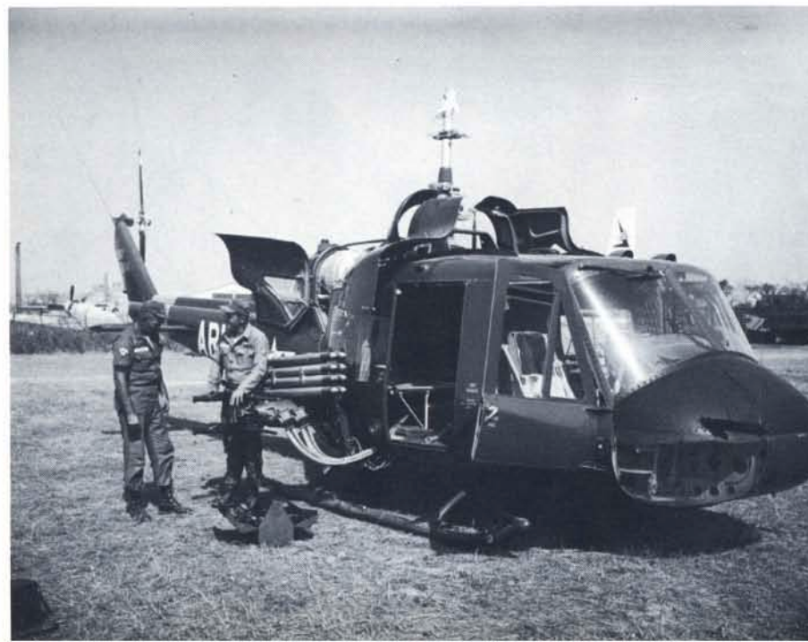
(Below) A brand new UTTCO UH-1B undergoes armament installation at Tan Son Nhut AB in Vietnam during February of 1963. The Huey mounts a factory-installed 7.62 machine gun and a 2.75 rocket kit. The pilot's seats were later replaced by armored versions. (US Army)
