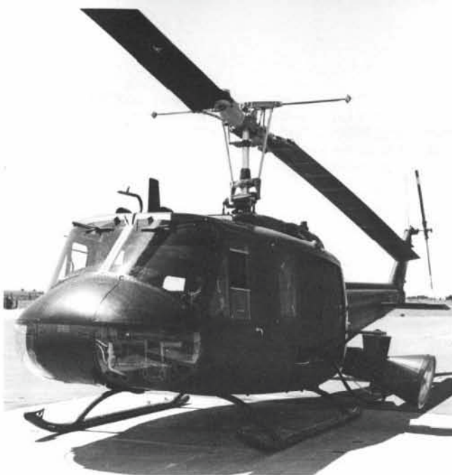
(Above) The Bell 'Night Sun' 20,000 watt xenon searchlight, fitted on a UH-1H, weighed nearly 300 pounds and could bathe a 900 foot circle on the ground in light from 3,000 feet. (Bell)
