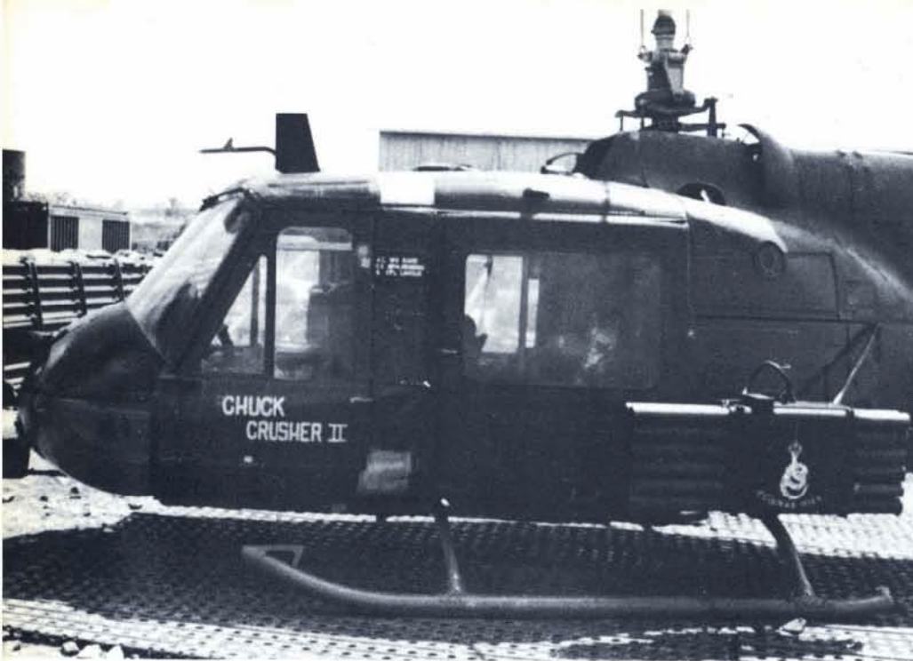
(Above) UH-1C Huey Hog of the 3rd Platoon, 114th Assault Helicopter Company armed with an XM-3 2.75 inch rocket system. (Eugene Schwanebeck)
