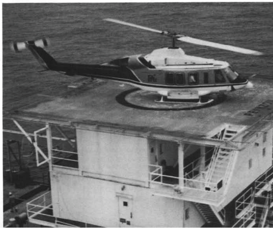
(Below Left) Though still a Huey, the 214ST bears little resemblance to the original design. This version can carry seventeen passengers plus the pilots. PHI operates a number of these for offshore oil work. (PHI)
