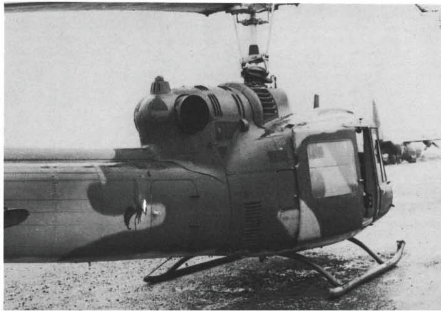
(Below) When the General electric T-58 engine replaced the Lycoming engine the exhaust was re-routed out the starboard side of the Airforce UH-1F variants. For rotary clearance the D model tail boom was used that had a two bay baggage compartment built into the starboard side. The Green Hornet emblem was found only on 20th SOS UH-1F and P Hueys. (Bob Chenoweth)
