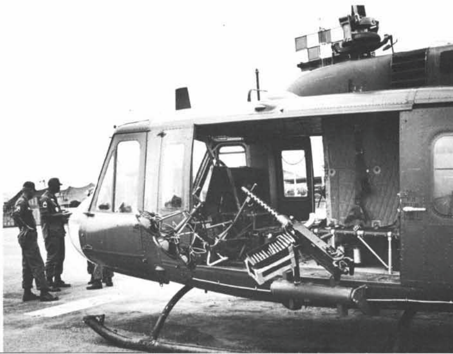
(Below) UH-1D Nighthawk Huey at Tan Son Nhut in January of 1967 with a 'Lightning Bug' searchlight backed up by a .50 caliber M-2 system (US Army)
