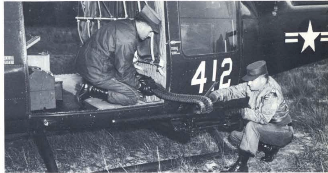
(Above) An experimental .50 caliber machine gun system mounted on a UH-1A of the 1st Armored Division is being loaded at Ft. Stewart's Metz Firing Range in late 1962. (US Army)
