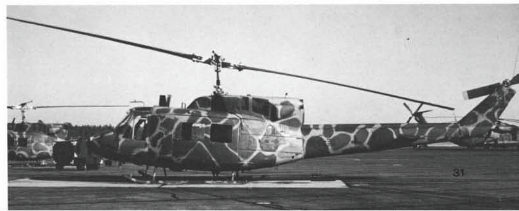
(Below) One of five UH-1Ns used by the USAF's obscure 20th Special Operations Squadron (SOS) at Hurlburt Field, FL. The non-standard camouflage of Light Green, Dark Green, and Light Brown segmented by Light Gray continues onto the skids. Like their ancestors of the Vietnam war, these Hueys bear a minimum of markings and carry the same 'Green Hornet' emblem on the tail boom. Early 1982. (Mike Campbell)
