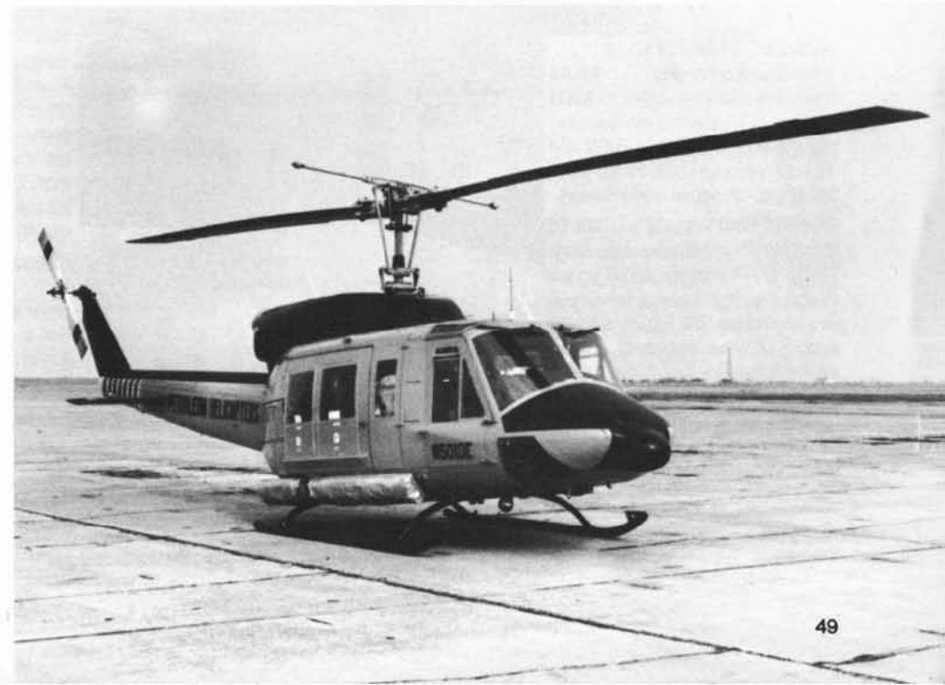
(Below Right) This PHI owned Bell 212 Twin in the PHI livery of Yellow and Black, carries inflatable floats on the lower sides of the fuselage and weather radar in the nose. (Boyd Waechter)
