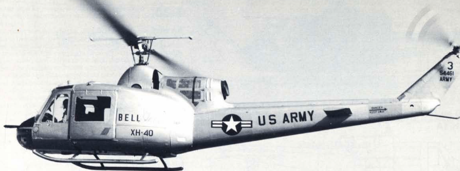
(Below) This YH-40, one of six evaluation machines built, clearly exhibits the significant improvements made over the XH-40 prototype — including the addition of the Bell-developed stabilizer bar mounted above the main rotor, a redesigned air intake and transmission cowling, and the relocation of the synchronized elevators to a more forward position on the tail boom. (Bell)
