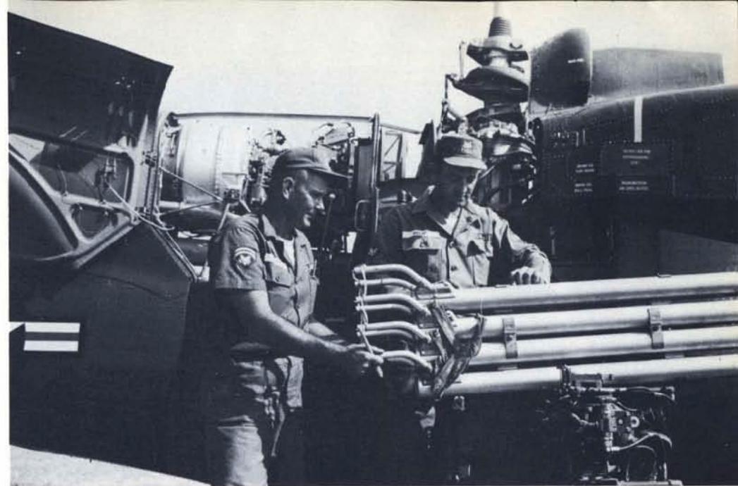
(Above) Installation of the 2.75 inch rocket kits could be done quickly and easily, and provided tremendous firepower to the Huey. (US Army)
