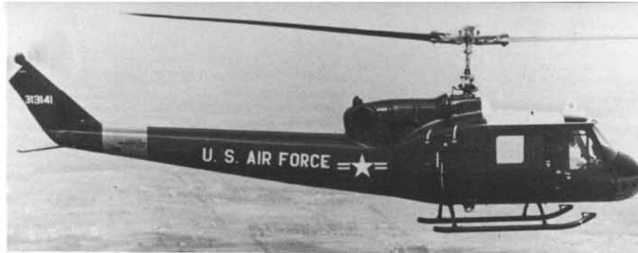
(Above) Officially called the H-48 in the USAF designation system, this was the first of 119 UH-1Fs delivered to the Air Force. Overstocked GE T58 engines were mated with the short-bodied airframe resulting in an unusual exhaust configuration. (US Air Force)
