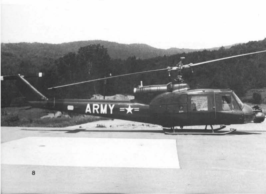
(Below) A UH-1A was fitted with an XM-5 40mm grenade launcher for tests at Springfield Armory in 1962. (US Army)
