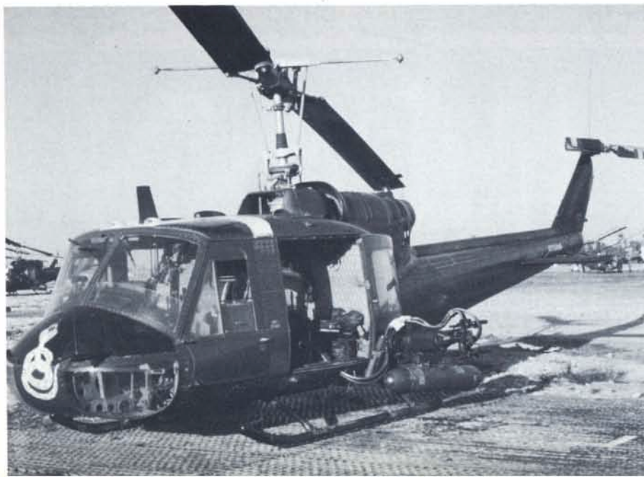
(Below) The 'gun' platoon of the 114th Aviation Company at Vinh Long, Vietnam used UH-1B Hueys in 1965. This example carries the unit markings of a Cobra on the nose. The White roof area aided in recognition from above. An XM-6 quad machine gun armament system is mounted along with a makeshift smoke grenade 'drop tube'. Eleven Purple Hearts are visible on the door post. (Charles Counts via Geneva Warren)
