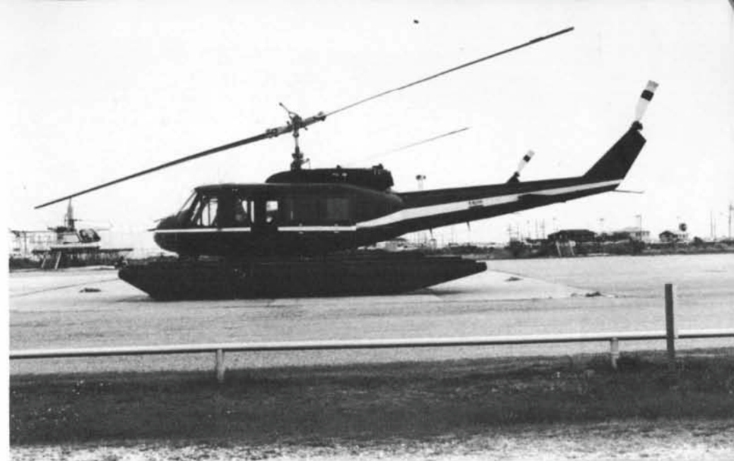
(Above Right) Bell 205A-1 in Red and White lower surfaces, and Black upper surfaces in 1983. This Exxon owned float Huey had its tail rotor on the right side. (Boyd Waechter)
