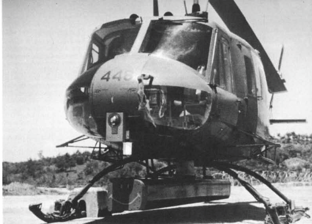
(Above) The high skid gear on the JUH-1 Stand-off Target Acquisitions System (SOTAS) retracted to allow rotation of the AN/APR 94 radar boom which had a frowning face painted in yellow on the opposite end. Though configured as an 'H' model, this Huey retains the pitot tube on the nose. Note the boarding step block over the starboard skid. Number 448 is seen in Korea during May 1976. (US Army)
