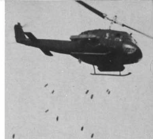
(Above) A UH-1H of the 101st Airborne Division sowing mines from bomb dispensers during 'Reforger 76' in Germany. (US Army)
