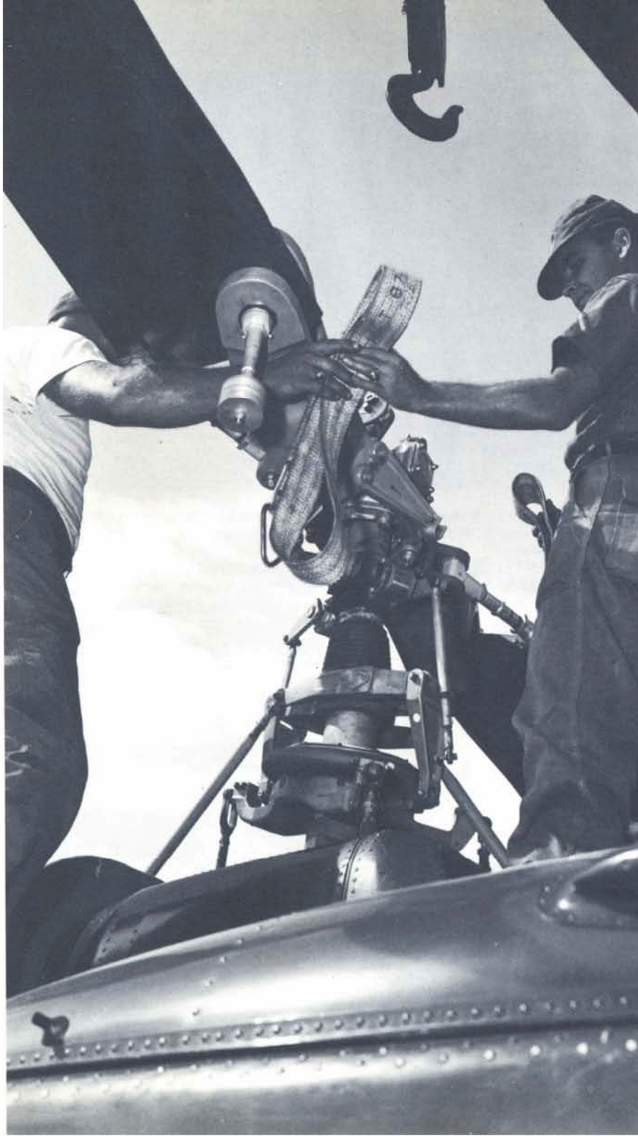
(Left) A UH-1A of UTTCO undergoes a rotor head replacement at Tan Son Nhut on 28 November 1962. (US Army)
