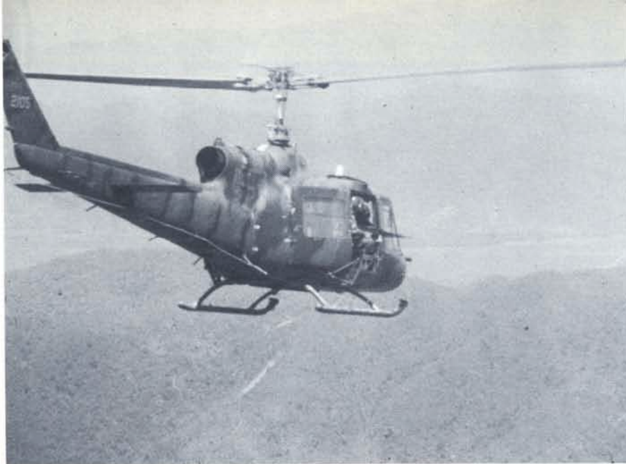
(Above) Early in the Vietnam war, Army aviation units experimented with a variety of camouflage schemes. This pattern of Gloss Black and Light Brown over Olive Drab was unique to the UH-1Bs of the 117th Aviation Company in 1964. HF antennas can be seen on both sides of the tail boom. (Cary Shelton)
