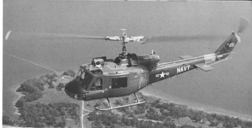
(Above) The first of the eight UH-1Ls built flies over Texas. This Huey exhibits the 'C' model characteristics which include a cambered tail fin, asymmetrical elevators, screened air intake section, and fuel filler on the port side. This aircraft was destroyed in a crash at Binh Thuy, Vietnam in late 1970. (Bell)
