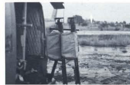
(Below Left) These 'piggyback' M60 machine guns, provided the firepower necessary for a 'chase' ship to rescue downed aircrews in Vietnam. (Author)
