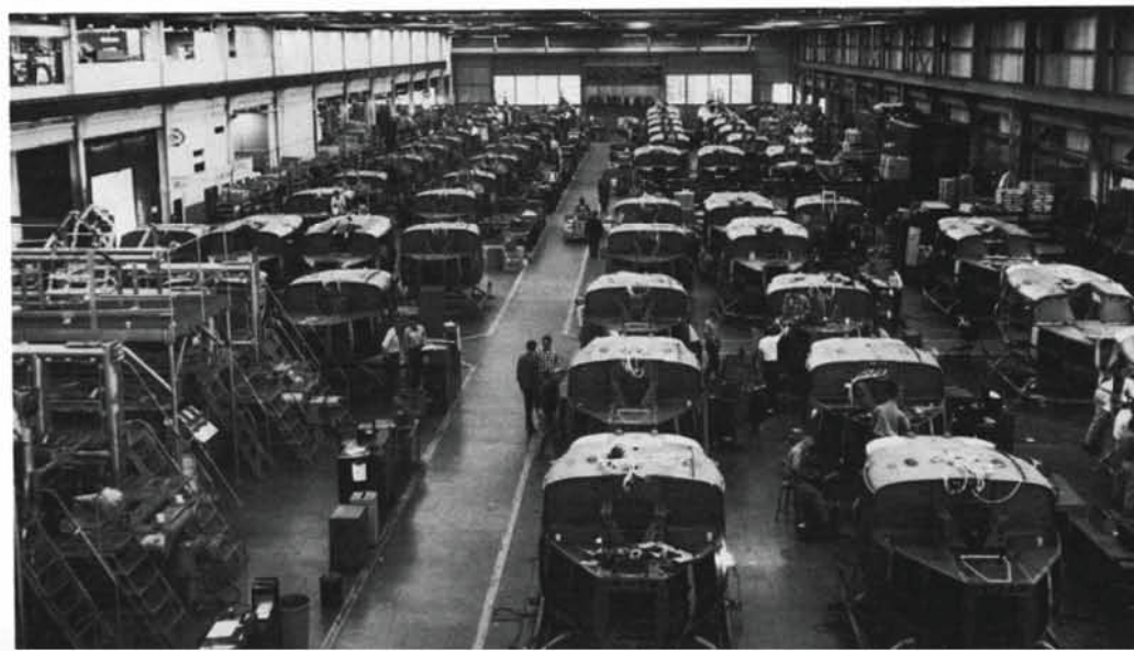
(Below) The Bell production line at Hurst, Texas is filled with Hueys still in the early stages of construction. (Bell)
