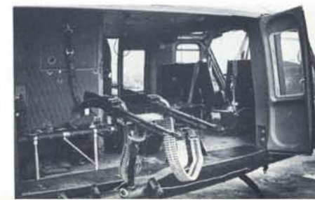
(Below Right) This makeshift arrangement of twin M60s was installed in a UH-1D at Tan Son Nhut in 1967. (US Army)
