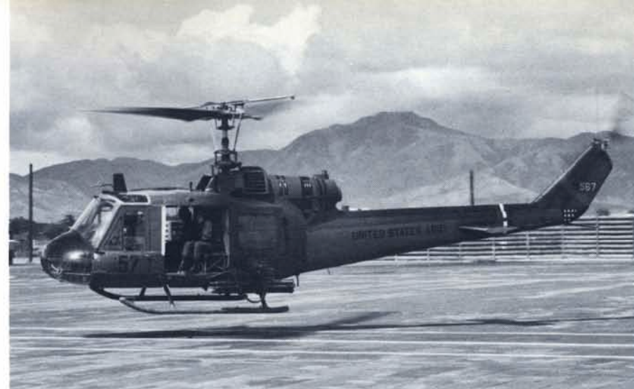
(Above) A UH-1C of the 57th AHC Cougars at Phu Cat. Designed specifically as a gunship the UH-1B was capable of carrying a wide variety of armament and is considered by many to be one of the great innovations of the Vietnam War. (Norm Taylor)
