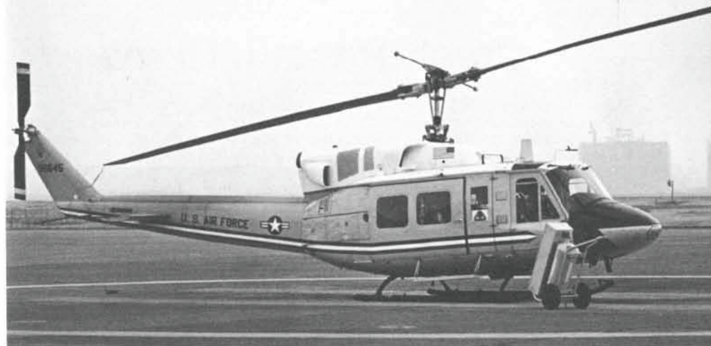
(Above) One of two UH-1Ns used by the USAF 475th Air Base Wing at Yokota AB, Japan in 1979/80. These twin engine Hueys were finished in Light Gray with White Roofs and Red, White, and Blue trim. (US Air Force)
