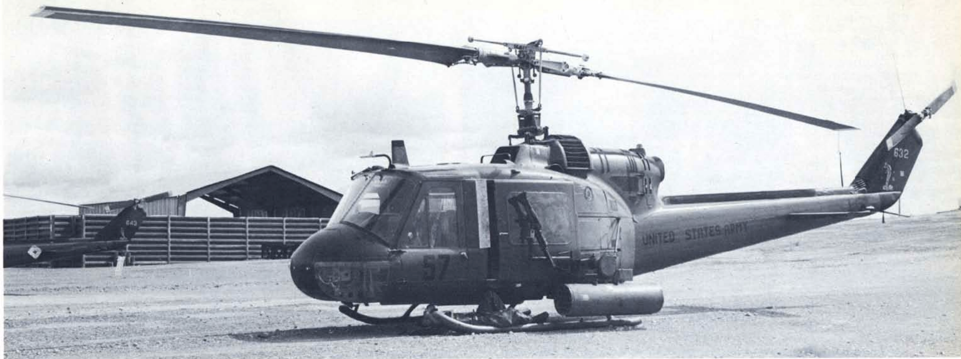
(Above) This UH-1C carries markings from two different units in Vietnam nullifying any attempt at identification — evidently the pilot's door came from the 57th Assault Helicopter Company (AHC), and the Cobra on the tail fin was used by the 129th AHC. This gunship at Phu Cat in 1971 mounts XM-159 rocket pods and an early type M60 Sagami mount. A wind baffle has been attached to the door post. The diamond on the Huey in the background was carried by any number of units. (Norm Taylor)
