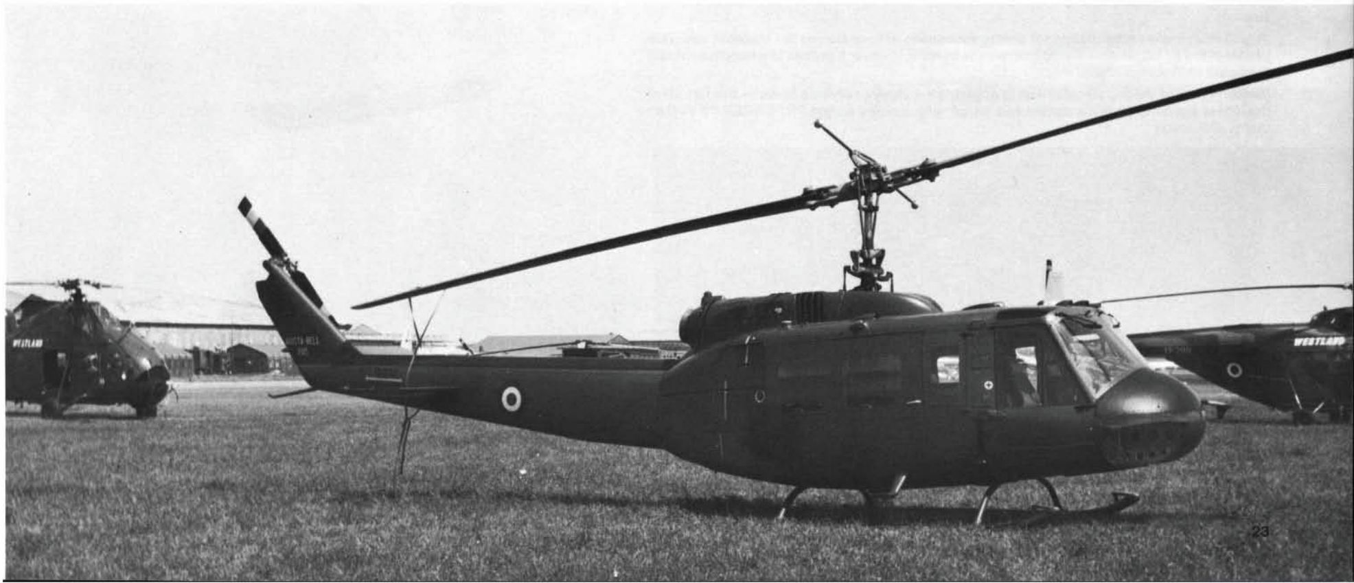
(Below) A factory fresh 205 produced under license in Italy by Agusta Bell. The Italian stencils just aft of the synchronized elevators include the designation 'UH-1D'. The main rotor blade has been anchored to the tail boom to prevent movement by the wind. (Tom Hansen)
