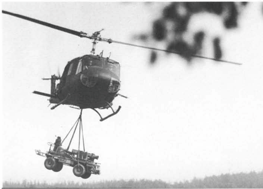
(Below) A UH-1H of the 101st Airborne (Air Assault) Division lifts a half-ton truck platform during 'Reforger 76'. (US Army)
