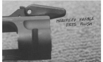
the metric. Each may be slightly different in dimensions. Scribe a line .300" from the front face of the receiver on the cocking slide channel. Using a rotary cutting tool or a grinder, hog-out material up to that line. Finish with a sharp file. Test fit with the weapon assembled and verify that the handle snaps into place.
