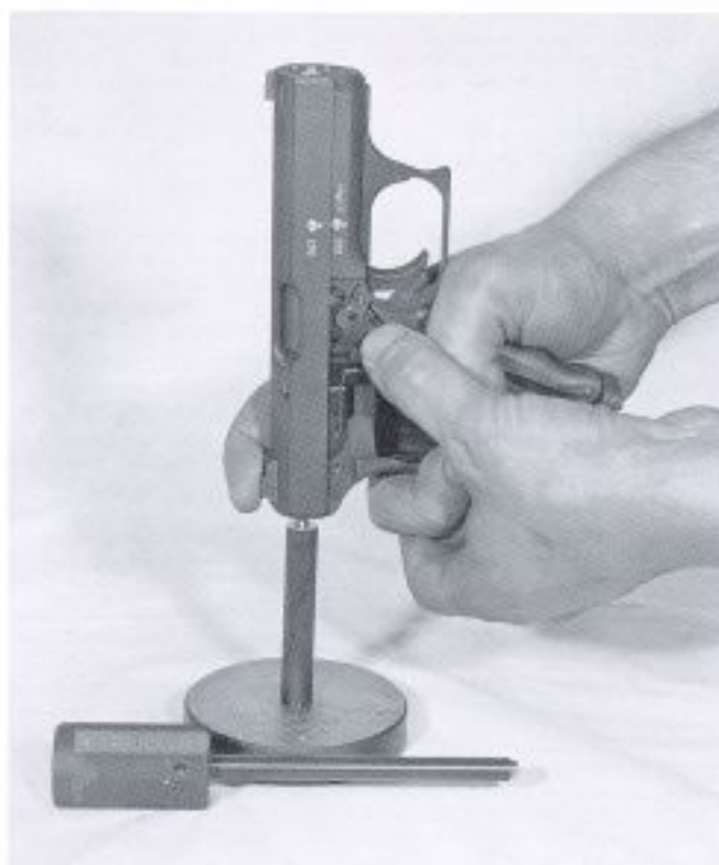
Figure 20. Inspection of firing pin front protrusion.
