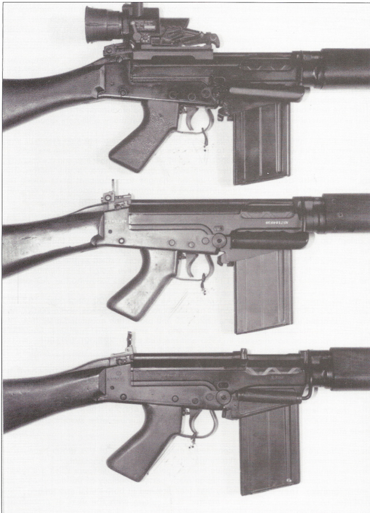
Top to bottom— 7.62mm L1A1 rifles of British, Australian and Canadian manufacture. UK makers' indicators are UE for Enfield, UB for BSA and UF for Fazakerley. The next rifle down is Australian production at Lithgow while the bottom example is a Canadian Long Branch. The Trilux SUIT sight fitted at top was an option. M.O.D. Pattern Room
