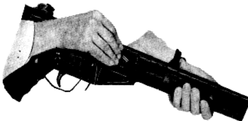
Fig. 56: Loading of propellant charge
