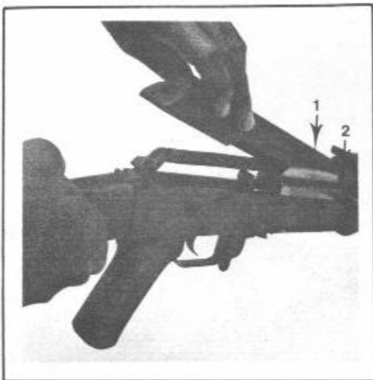
FIGURE 45. REPLACING BOLT COVER
