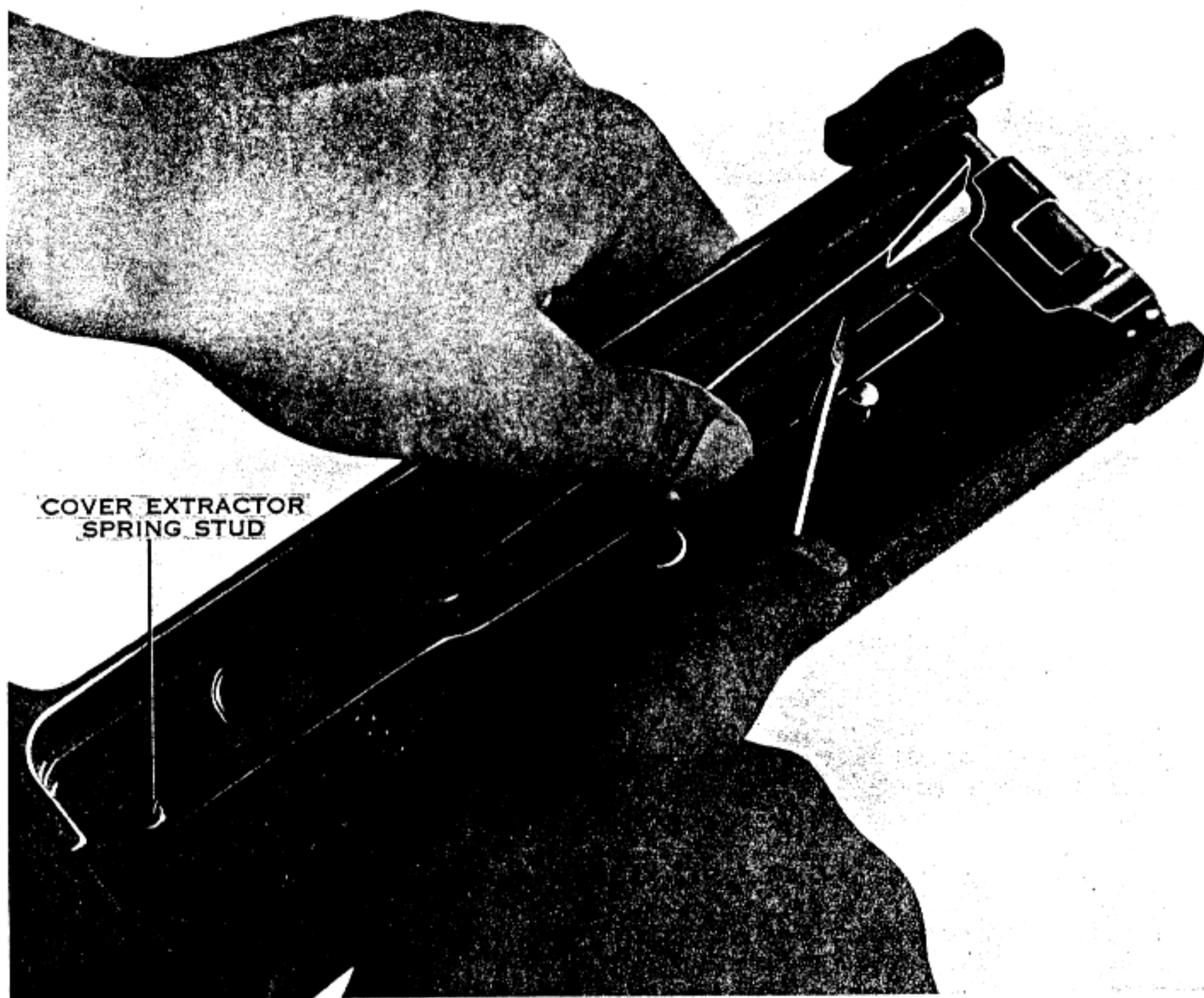
Figure 61. Removing the cover extractor spring.
