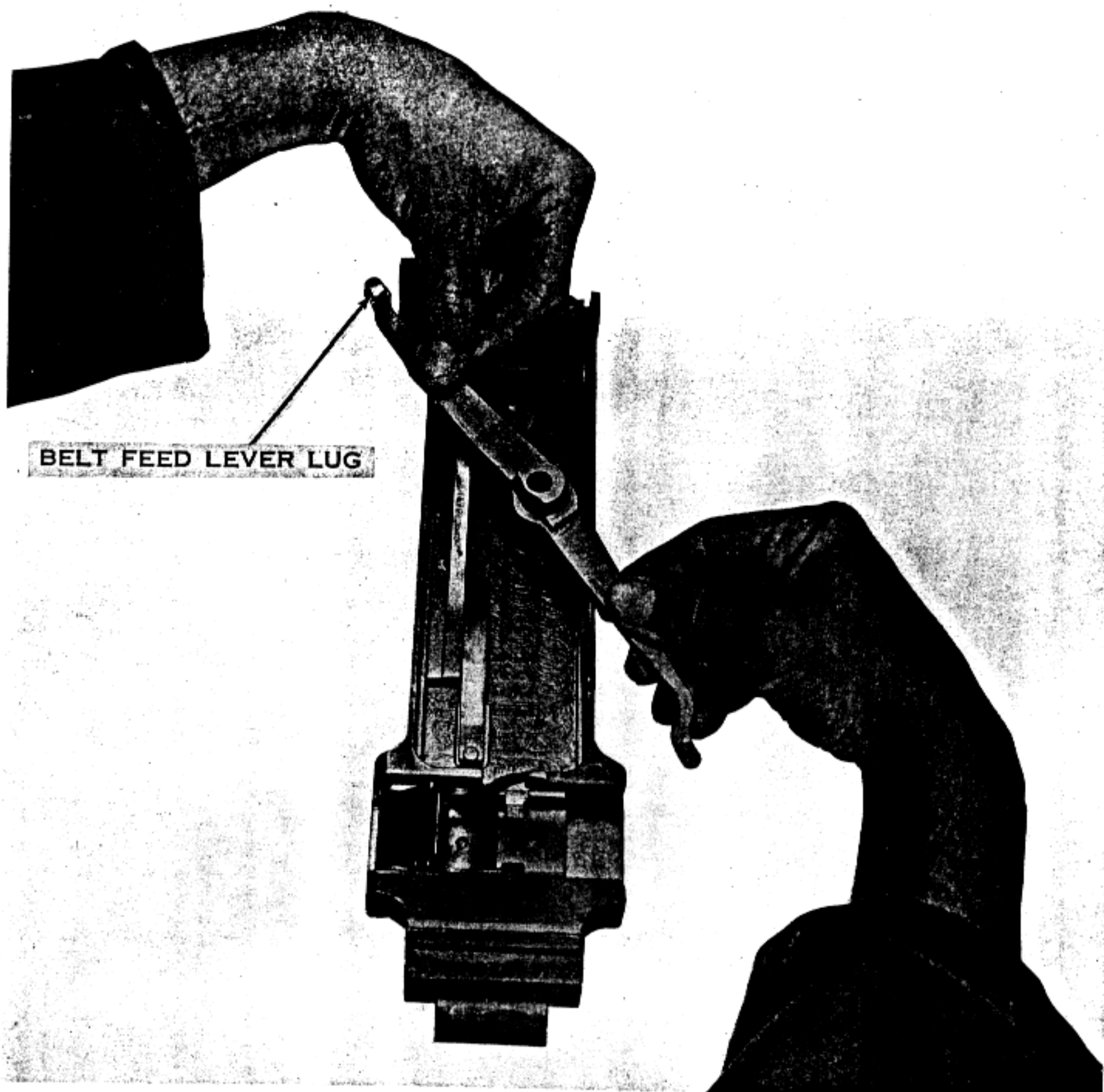
Figure 67. Placing the belt feed lever over its pivot stud.
