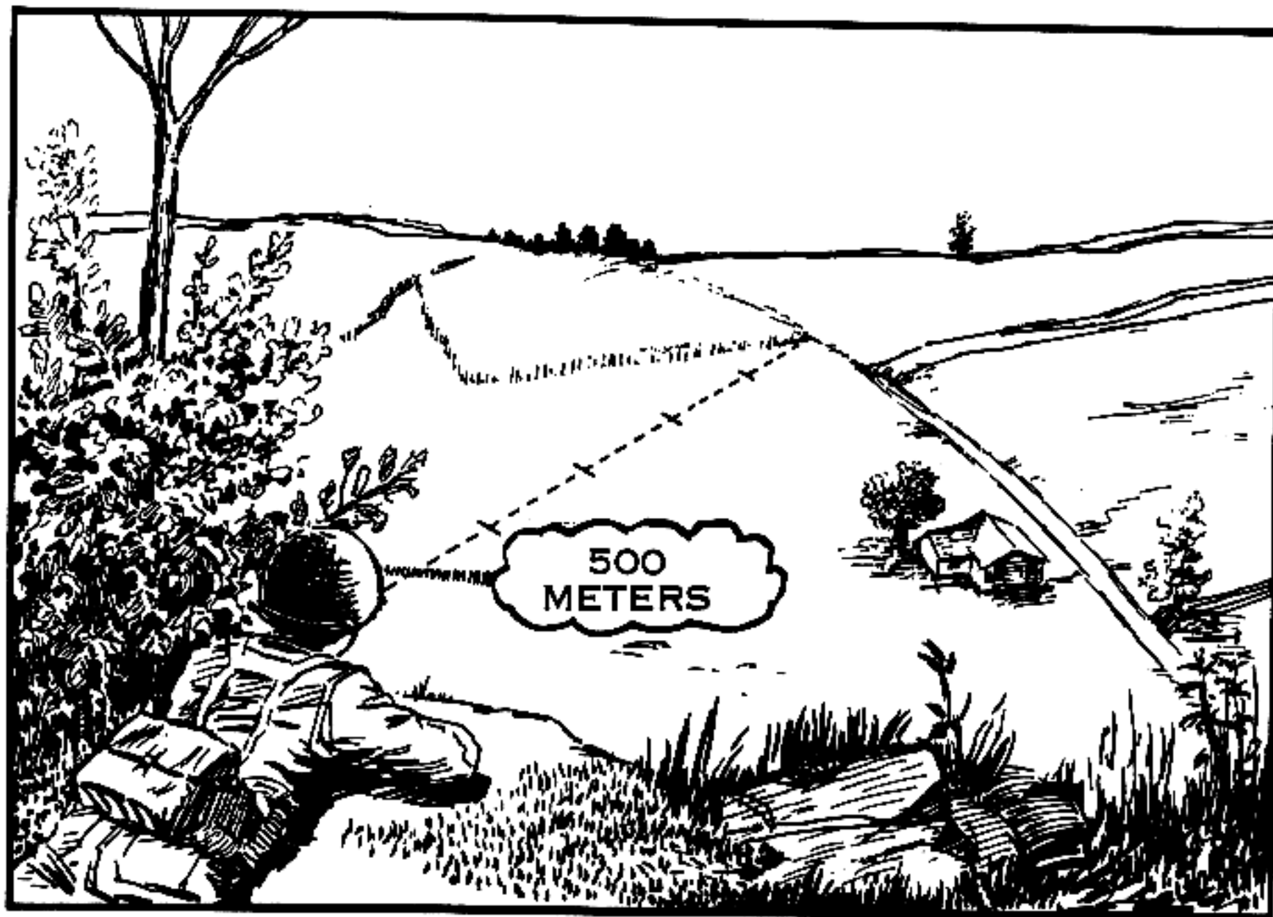
Figure 131. Applying the 100-meter unit of measurement method for ranges up to 500 meters.
