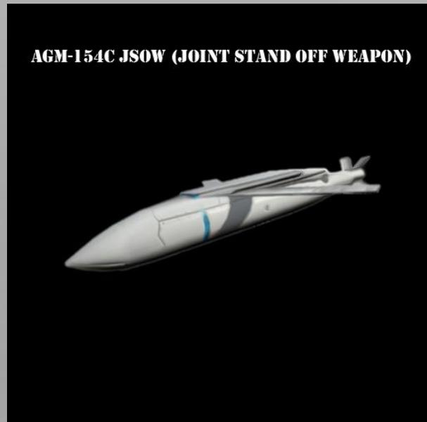
The AGM-154C, in addition to the common GPS/INS guidance, will use an autonomous imaging infrared seeker for target acquisition and terminal guidance. The JSOW-C incorporates a Raytheon-developed uncooled, long-wave infrared seeker with ATA algorithms, thus providing the Navy with a launch-and-leave weapon with standoff precision strike capability.
